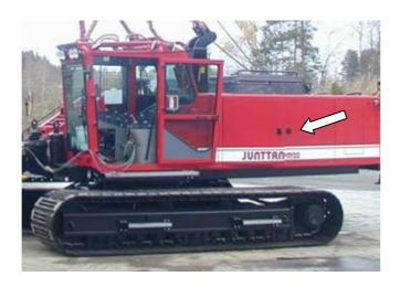
• The hydraulic oil level should be at least in the middle of level glass.
