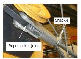
Pull the rope through the rope socket joint from the narrower side, make a loop and pull the rope back to the bushing. To prevent the rope from getting loose put the cotter to the rope socket and shackle on top of the cable as shown in the picture. After that, tighten the cable until the cotter locks without clearance.
