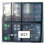
There are two signal lights on the top console which are important when lifting or lowering the leader.
