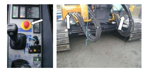
• Start the engine and test the function of each button in turns. Repair the damaged buttons immediately.
